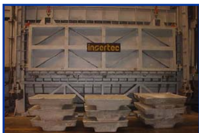
Dry-Hearth Reverb Furnace
