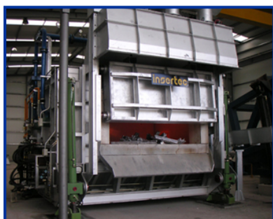
Tilting Reverb Furnace
