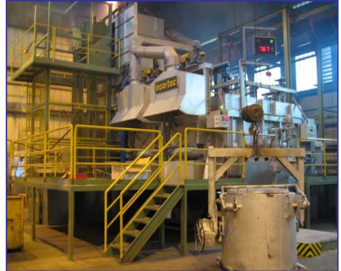
Combination MELTOWER Furnace with Skip elevator
