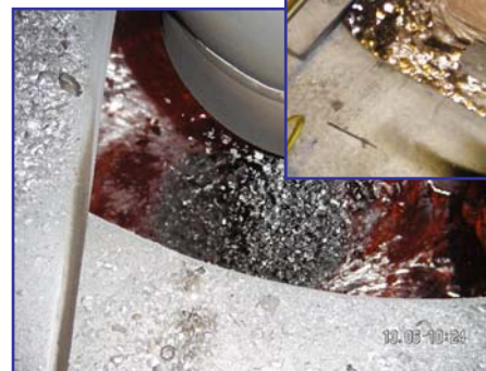
Sink Vortex Chamber with Chips entrainment
