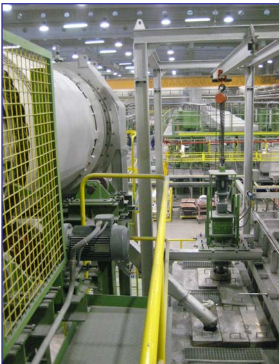
ALUSWIRLER chamber and feed of chips
