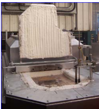
Ladling well with T/C and level sensor
