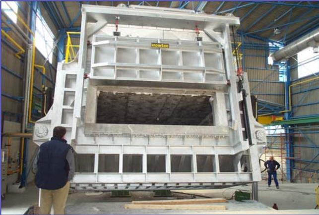
View of a tilted furnace with the door opened
