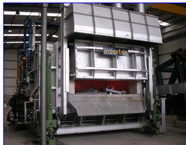
Detail of main doors with dry pre-cast shape frames
