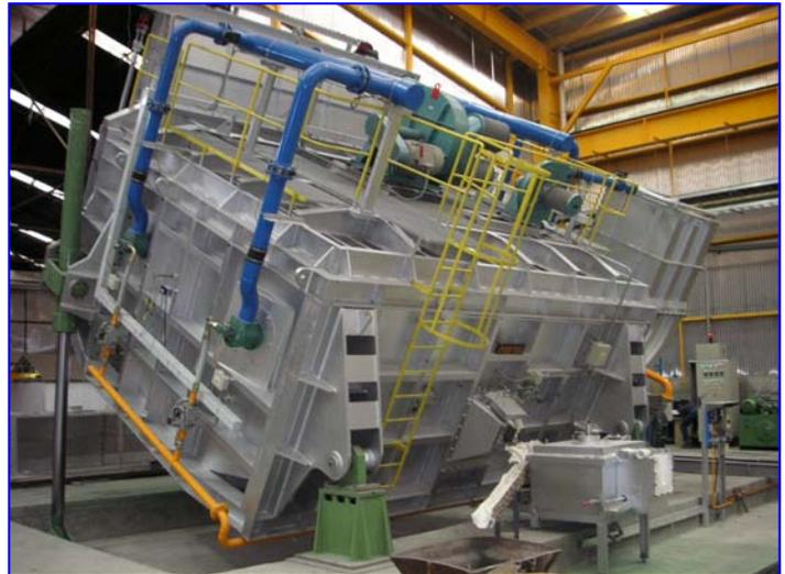
**Flat roof** fabricated from steel sections for added strength and the composite refractory lining is chosen for its thermal properties and durability .
