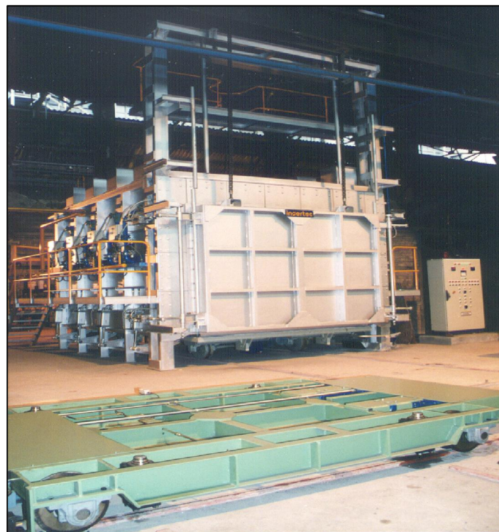
Front view of Bogie-hearth Furnace with bogie transfer car for handling on site.
