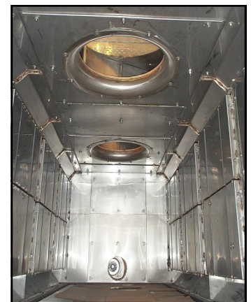
Furnace heating chamber inside view.
