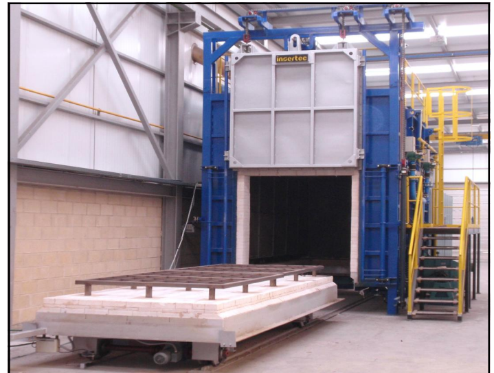
Bogie Hearth type Recirculation Furnace provided with sliding front door.
