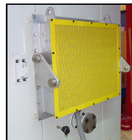
Heating elements assembly detail for easy access from the outside of Furnace .
