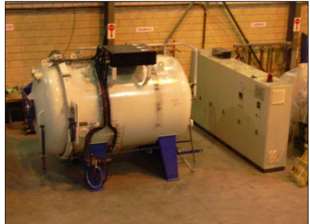
Horizontal-loaded Vacuum Furnace being preassembled at INSERTEC workshop.
