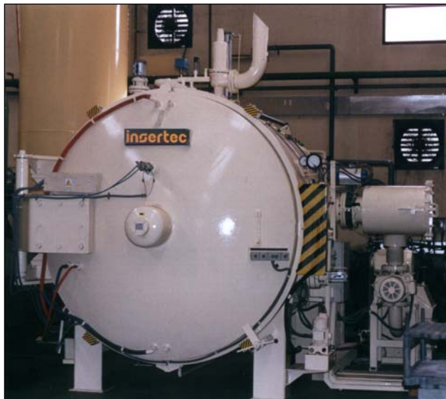
Horizontal-loaded Vacuum Furnace for Annealing and Tempering.
