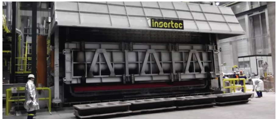
\ Tilting reverb furnace
