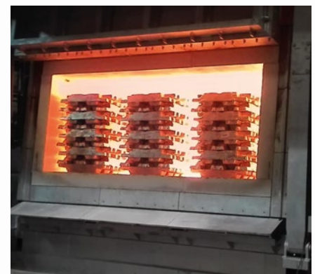
\ Dry hearth reverb furnace
