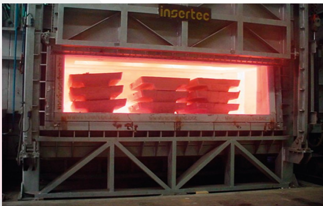
\ Dry hearth for ingot bundles or sows melting.
