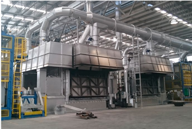
\ 35 Mton stationary sidewell melter.
