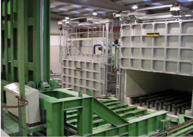
\ Chamber Furnaces provided with sliding front door.
