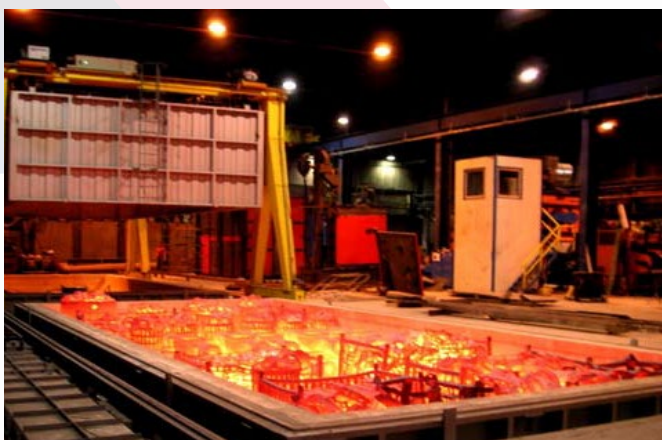
\ Travelling bell type chamber furnace provided with two load-unload bases.
