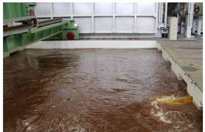
\ Quenching tank (water, oil or polymer).
